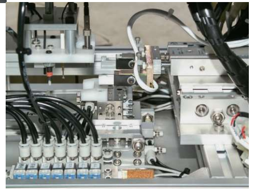
製罐の変形・不良検出 Detecting the deformation and/or defect of can
