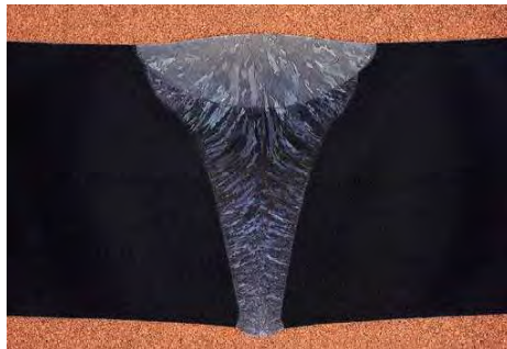
溶接の溶け込み
